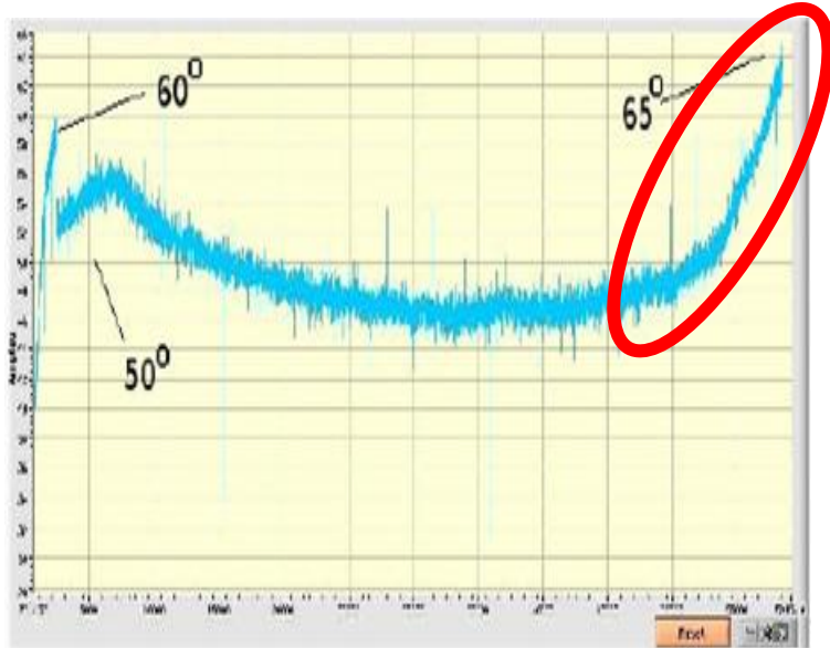
Rapid Temperature Rise Lubrication Failure
