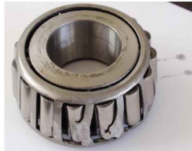
Entrapment Of Failed Cage
