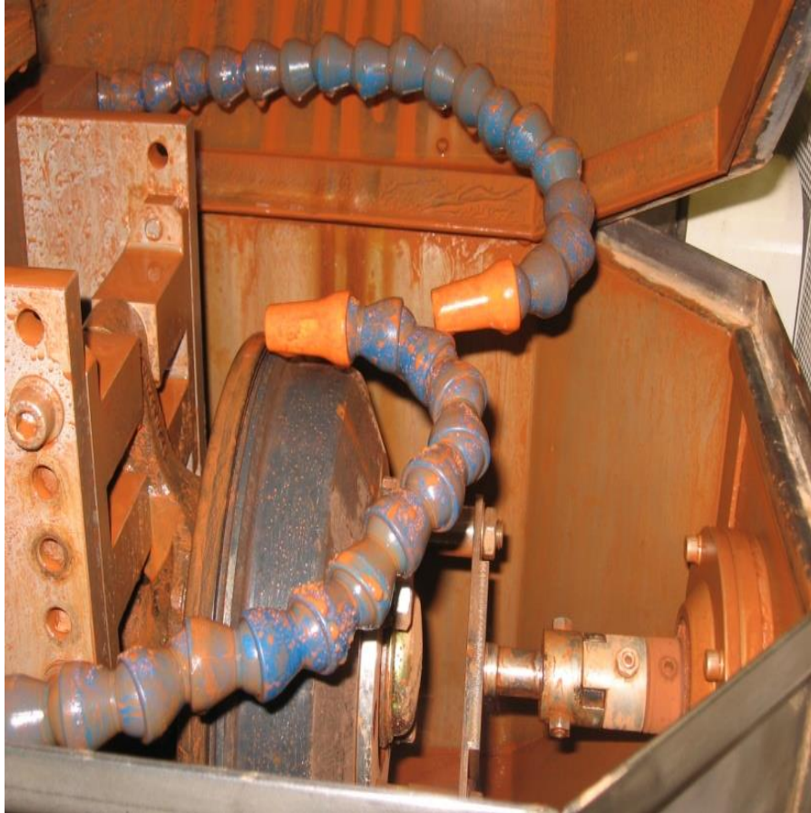
Hub Bearing Test With Mud Ingress Setup
